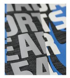
Seamless transfers are designed to eliminate excess printed area or key-line surrounding a complex logo. Whether it's detailed text or complex graphics, seamless transfers can be used to achieve a clean look with perfectly weeded out transfers.
